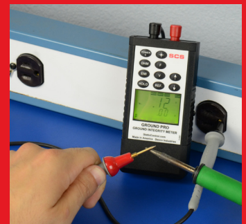
Measuring EMI Voltage on a Soldering Iron
