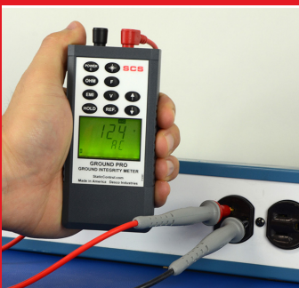
Measuring AC Voltage between Hot and Ground
