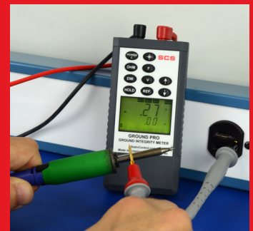
Measuring EMI Voltage on a Soldering Iron
