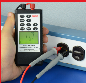
Measuring AC Voltage between Hot and Ground
