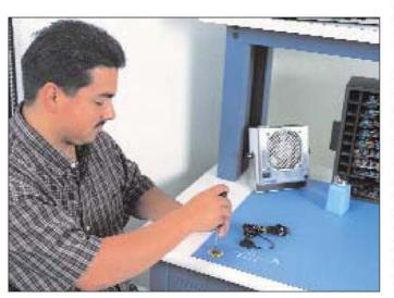
counterparts. The ESD dissipative characteristic is added so when charged conductors (conductive or dissipative) items are placed upon the surface a controlled discharge occurs and electrostatic charges are removed to ground. This occurs only if the ESD worksurface is actually connected to ground.
